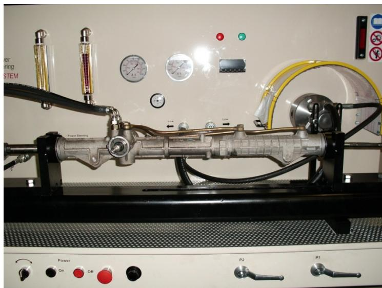
Connect the tie rod of the rack with the braking system.
