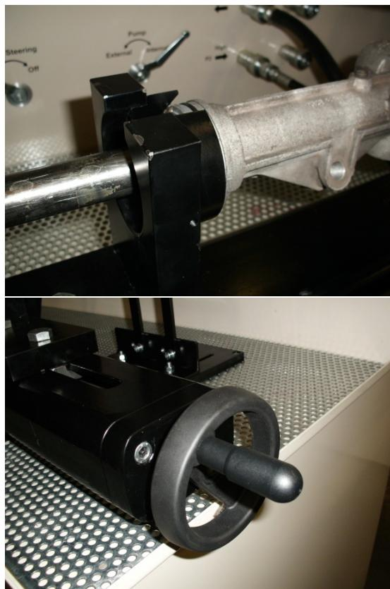
Close the two bolts of the right support. Remember that when you move the right support by means of the hand wheel you have to unscrew a little the bolts that lock the right support. After moving you have to close the two bolts.
