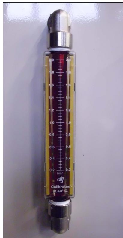
In the second flow meter you can see the total flow of oil into the hydraulic circuit.
