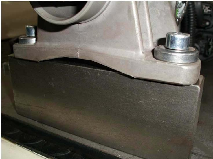
Assembly together the tool #1 (main plate) and the 2 pieces of tools #3 (vertical support for GolfV). Fit the EPS on the support locking it with M8 bolt.
