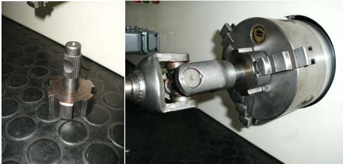
Screw the Tie rod (tool #14) to the EPS and to the Main Rack.
