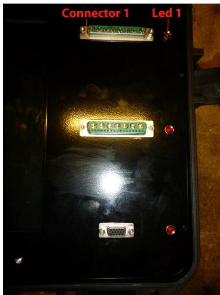
Now open the page of the model that you want to test and connect its cable into the 'connector 2' that is located below the battery connector. The Led 2 lights only after giving the Power Supply ON.
